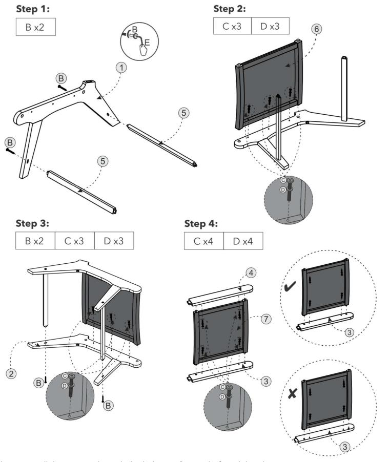
Please put all the screws through the holes on 2 parts before tightening. Holes may be covered by wicker. Please find spot mark on wicker if you can't find a hole to assemble.
