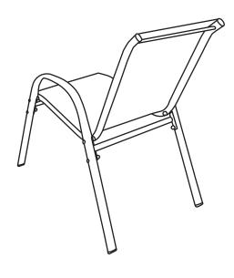
When fixing the seat to the other side of the legs, it can be easier to put the chair in a higher place, or lay the chair on the ground so you can see the fixings and stretch the textilene more easily.
