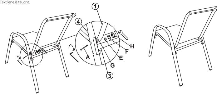
When fixing the seat to the other side of the legs, it can be easier to put the chair in a higher place, or lay the chair on the ground so you can see the fixings and stretch the textilene more easily.
