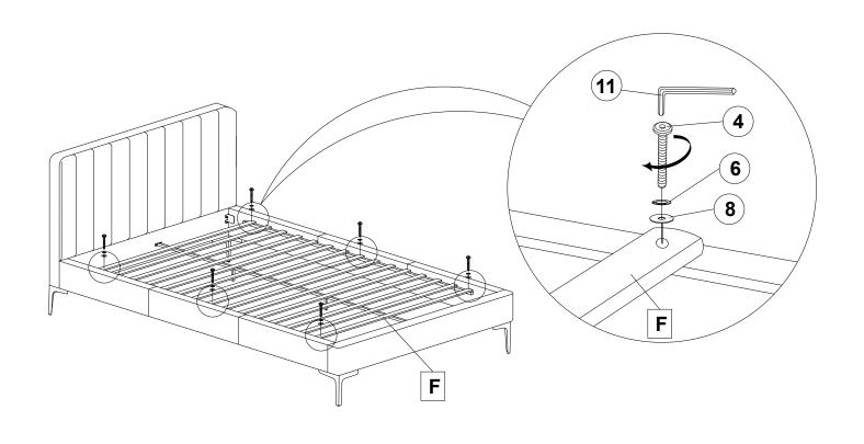
**Step 6**Assemble Slat (F) using CSK M4 x 30mm (10) with screwdriver as shown in figure.
