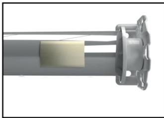
The illustration shows the fabric running off from the right hand side of the blind. To correct this, simply stick a small (30mm) strip of masking tape to the aluminium tube at the opposite end. Fully wind the blind up and then repeat until the fabric is no longer running off.
