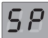
5. Push the bobbin to the right. When the bobbin winder spindle is pushed to the right, the screen will show "SP".
