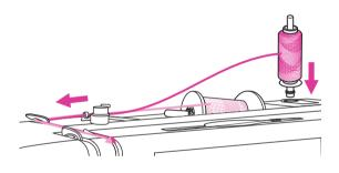
Follow the instructions for single-needle threading using the horizontal spool pin. Thread through the left needle.
