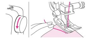
5. Turn the handwheel toward you (counterclockwise) to lower the needle into the fabric at the beginning of the stitching.
