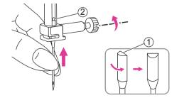
Inserting a 75/11 needle, keep the flat side of the shaft to the back.
