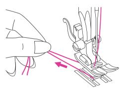
Pull both threads to the back under the presser foot.
