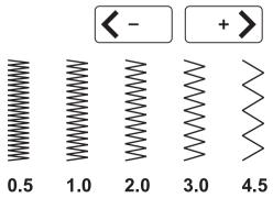
After selecting the stitch, touch the stitch length icon to enter the adjusting mode. Touch the value adjustment icon to adjust the stitch length.
