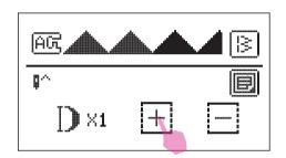
Touch the "+" or "-" icon to adjust the stitch which can be elongated up to 5 times the original length.
