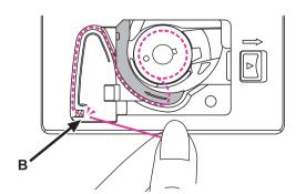
To cut off excessive thread, pull it to the cutter at point (B).
