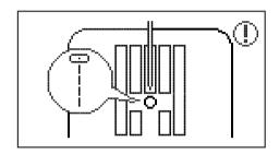
Only specific straight stitches are applicable while using straight stitch plate in sewing mode. (A group patterns 01 & 03 & 05)
