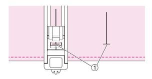
Position the fabric under the presser foot so that the centerline's mark is aligning with the center of the buttonhole foot.
