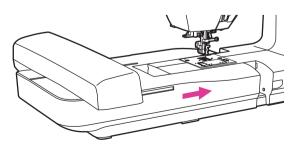
Slide the embroidery unit onto the machine arm. Push lightly until the unit clicks into place.
