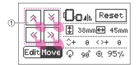
Touch the change position icon to change its position. A short touch will move one unit per time and a long touch will move 5 units per time.
