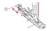
Extend the button holder plate and set to the desire length. Adjust the stitch width and the stitch length to the desired width and density.
