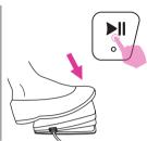
Hold the thread tail securely in one hand. Step on the foot control (only in the sewing mode) or long press the start/stop button to start winding the bobbin.
