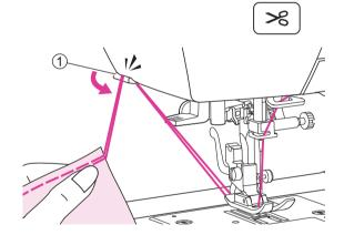
9. Press the thread cutter button to trim the threads.
