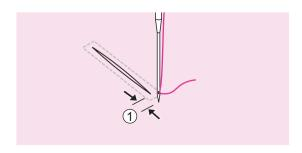
Position the fabric so that the needle is 2mm in front of the area to be darned, and then lower the presser foot lifter.
