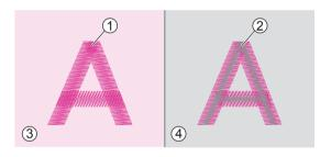
The thread tension is correct when upper thread is just visible on back of the fabric.
