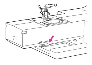
The drop feed lever can be seen on the base at the front side of the sewing machine, when the sewing table is opened.
