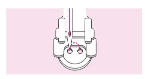
Select the buttonhole sewing stitch and adjust the stitch width according to the distance between the two holes of the button.
