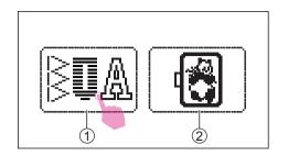
Turn the power switch to on ("I"). Touch the sewing mode icon.
