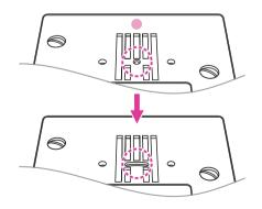
Replacing the straight stitch plate to normal needle plate.
