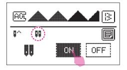
Touch the ON icon to set the twin needle function then the LCD screen will display the twin needle icon.
