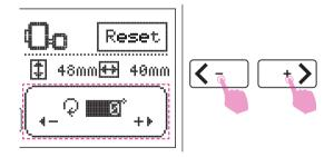
The screen will show the rotation option. The default is in 0 degree, and you can touch the value adjustment icon to rotate selected pattern clockwise or counter-clockwise.
