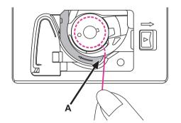
Pull the thread through the slit (A).
