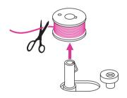
9. Cut the thread and then remove the bobbin.
