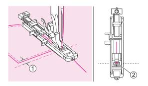
Position the fabric so that the needle is 2mm in front of where you want the sewing to start, and then lower the presser foot lifter.
