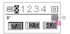
To adjust the stitch width, stitch length, and tension. Touch the setting icon to enter or exit the pattern fuction sceen.
