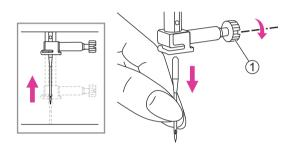
Turn the handwheel toward you to raise the needle then loosen the needle clamp screw to remove the needle.
