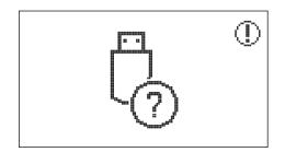
This machine can't save the embroidery pattern loaded from the USB stick. Please do not remove USB while the machine is in the editing or embroidery process, otherwise it will lead to data loss. An alarm screen will pop up if you remove the USB stick.
