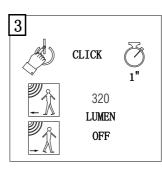
After mode 2, press the switch to change to mode 3. Product will be 320Lm when motion is detected and will turn off after 25 seconds.
