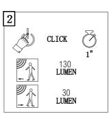
After mode 1, press the switch to change to mode 2. Product will stay on at 30Lm and increase to 130Lm when motion is detected (This will stay at 130Lm for 25 seconds then dim to 30Lm and stay lit).
