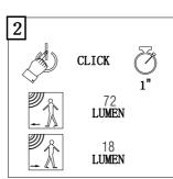
After mode 1, press the switch to change to mode 2. Product will stay on at 18Lm and increase to 72Lm when motion is detected (This will stay at 72Lm for 25 seconds then dim to 18Lm and stay lit).
