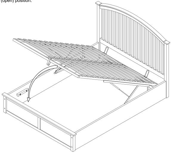
Lift with the strap (H12) and close with the strap. The strap should always be accessible. Take care not to lean over the bed when lifting, if the mattress is thin and light, the frame may rise quickly. The speed of closing will also depend on the weight of the mattress so always keep fingers well clear of the metal frame.
