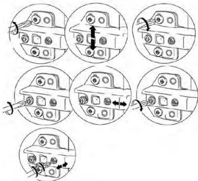
The door gap can be adjusted by regulating the hinges and the foot Levelers.
