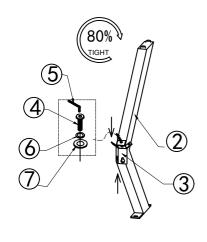
Note: DO NOT fully tighten bolts until unit is fully assembled and all bolts are in place.
