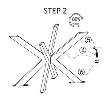
Note: DO NOT fully tighten bolts until unit is fully assembled and all bolts are in place.
