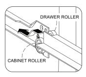
• Locate both roller on drawer box and roller on cabinet.
