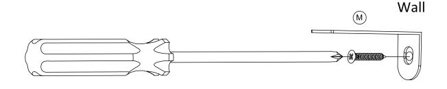
Secure the wall brackets (M) to the wall using screws (not included). Tighten with the screwdriver.
