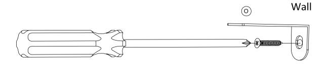
Secure the wall brackets (O) to the wall using screws (not included). Tighten with the screwdriver.
