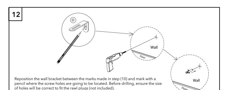
**Warning**: Ensure the area to be drilled is free from hidden electrical wires, water and gas pipes. **Caution**: The wall fixings supplied are for solid brick walls only.
