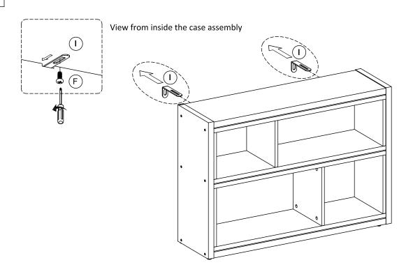
Loosen the screw (F) and remove the wall bracket (I) from the case assembly with screwdriver.
