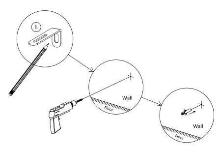
Reposition the wall bracket between the marks made on step (20) and mark with a pencil where the screw holes are going to be located. Before drilling, ensure the size of holes will be correct to fit the rawl plugs (not included).
