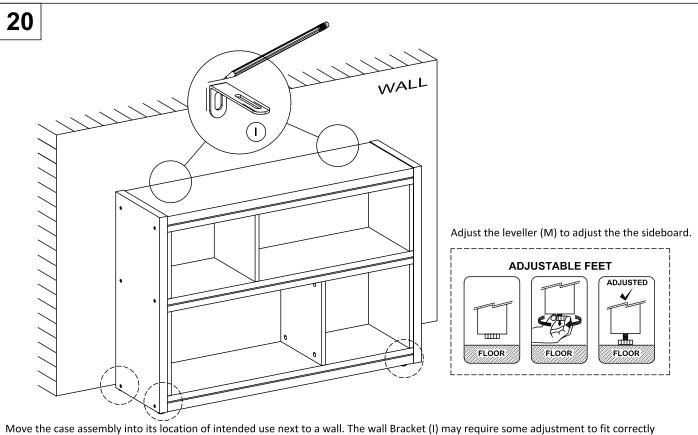
With a pencil lightly and precisely mark the position of the brackets on the wall. Now carefully move the cabinet away from the wall to allow
