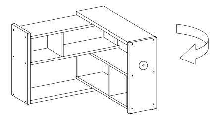
Turn forward 90° the assembly large right panel (4) to form a right-angle as shown.
