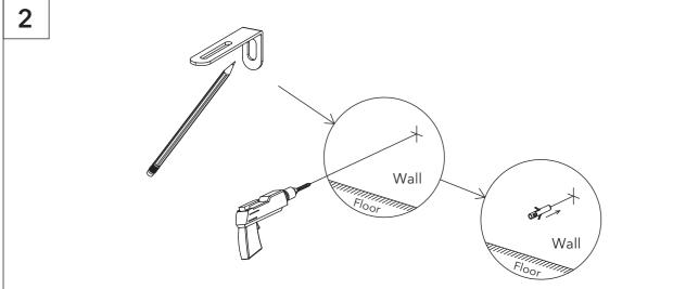
Move the furniture into its location of intended use against a wall. With a pencil lightly and precisely mark the position of the brackets on the wall. Carefully remove the furniture from the wall to allow space for drilling.
