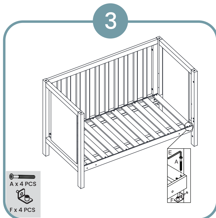
Assemble mattress using 4 x A bolts with 4 x F mattress base support
