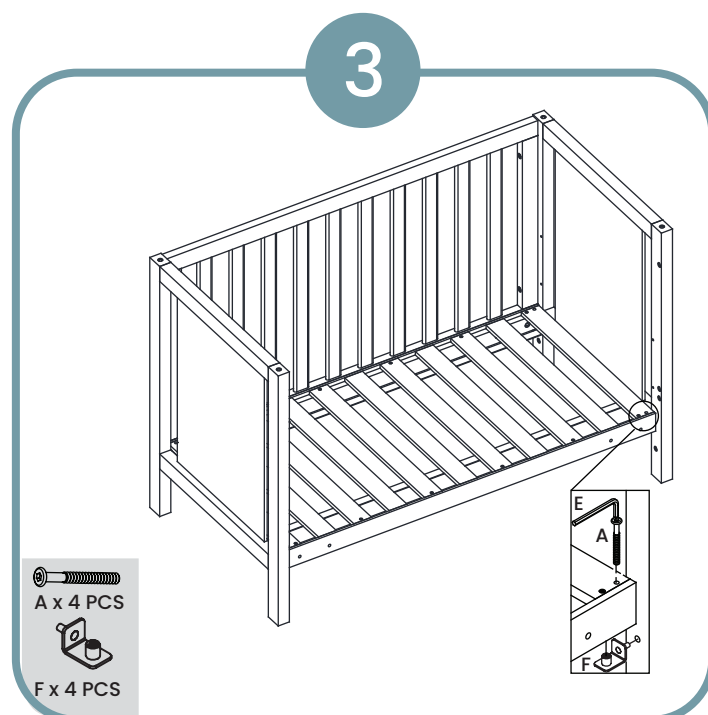
Assemble mattress base using 4 x A bolts with 4 x F mattress base support
