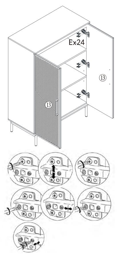
The gaps around door can be adjusted by loosening or tightening the screws on the hinges.
