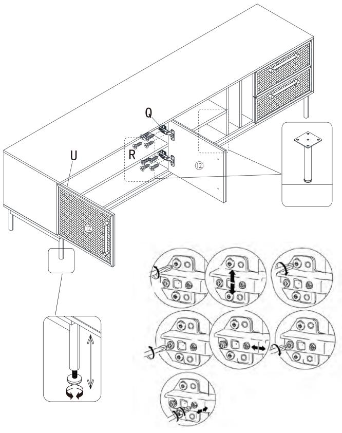
The gaps around door can be adjusted by loosening or tightening the screws on the hinges.
