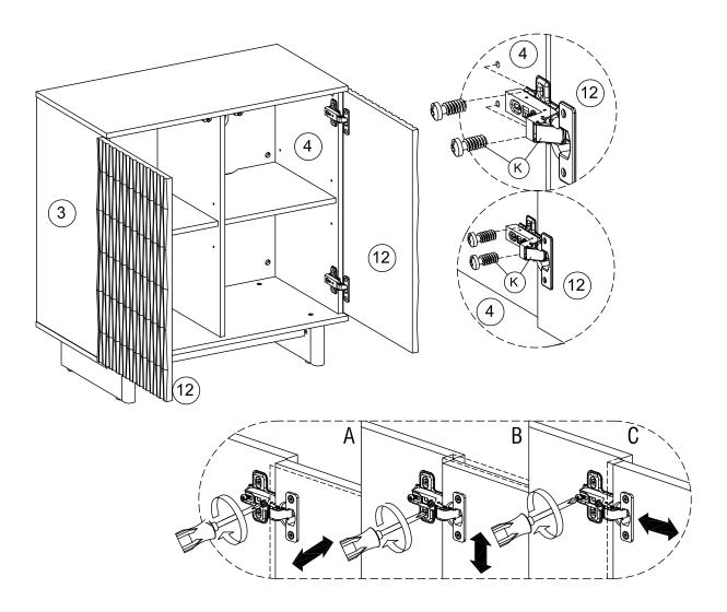
Attach the door (12) to cabinet as shown. Adjust the door until fix.
