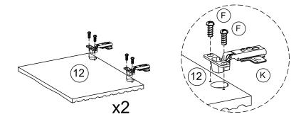
Install door hinge (K) to door (12) using screws (F).
