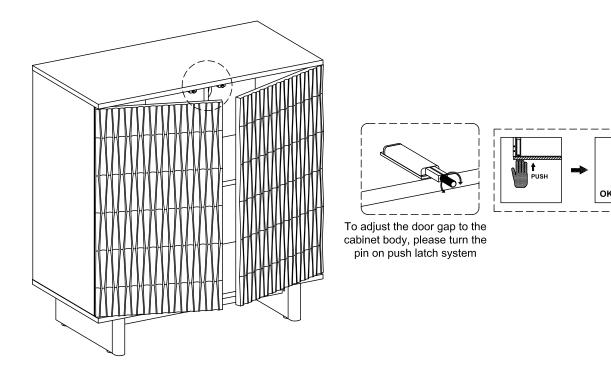
Adjust push latch (P) until fix with the door.
