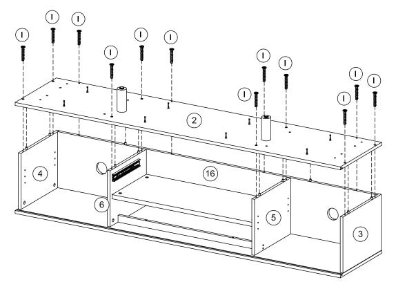
Attach bottom assembly to the case assembly using screws (I) as shown.
