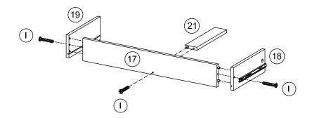
Attach left drawer (18), right drawer (19) and bottom support drawer (21) to rear drawer (17) using screws (I).
