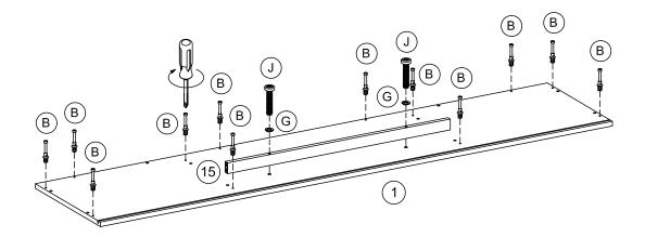
Attach cam-bolt (B) to top panel (1) using screwdriver. Attach metal support (15) to top panel (1) using screws (J) and washer (G) as shown.
