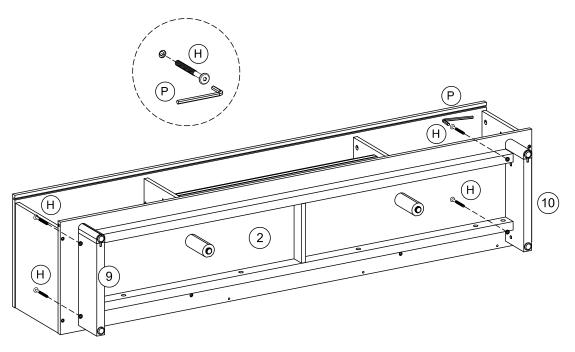
Tighten assembly bottom support with base panel (2) using screws (H) and allen key (P).
