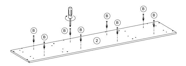
Attach cam-bolt (B) to Base panel (2) using screwdriver.
