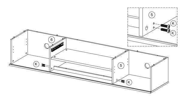
Tighten the metal support with divider panel using screws (K).
