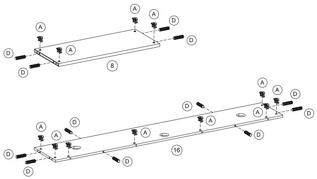
Insert cam-lock (A) and dowel (D) into middle panel (8) and rear panel (16).
