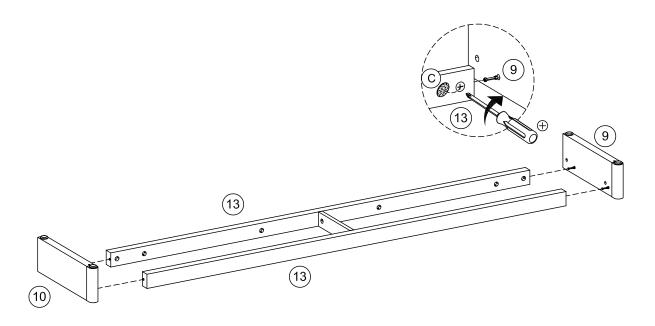
Attach left leg (9) and right leg (10) to bottom large support (13) as shown. Turn the cam-lock (A) clockwise to lock using screwdriver, then paste cam-sticker (C).
