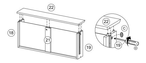
Attach front drawer (22) to the drawer assembly as shown. Turn the cam-lock (A) clockwise to lock using screwdriver, then paste cam-sticker (C).
