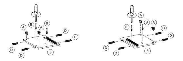
Attach cam-bolt (B) to left divider panel (5) and right divider panel (6) using screwdriver. Insert cam-lock (A) and dowel (D) into left divider panel (5) and right divider panel (6).
