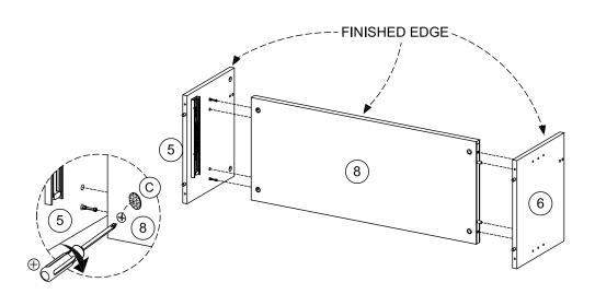
Attach Left divider panel (5) and Right divider panel (6) to middle panel (8) as shown. Turn the cam-lock (A) clockwise to lock using screwdriver, then paste cam-sticker (C).
