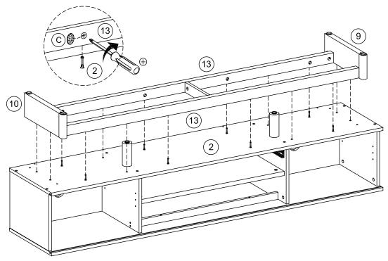
Attach assembly bottom support to base panel (2) as shown. Turn the cam-lock (A) clockwise to lock using screwdriver, then paste cam-sticker (C).
