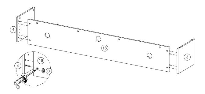
Attach left panel (3) and right panel (4) to rear panel (16) as shown. Turn the cam-lock (A) clockwise to lock using screwdriver, then paste cam-sticker (C).
