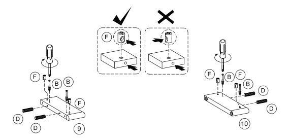
Attach cam-bolt (B) to left leg (9) and right leg (10) using screwdriver. Insert barrel nuts (F) and dowel (D) into left leg (9) and right leg (10).
