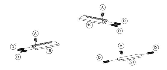
Insert cam-lock (A) and dowel (D) into left drawer (18), right drawer (19) and bottom support drawer (21)..
