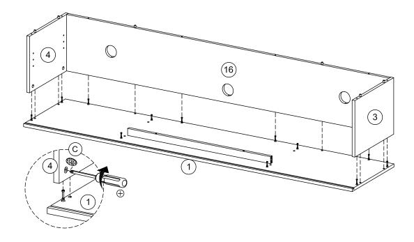
Attach case assembly to top panel (1) as shown.
