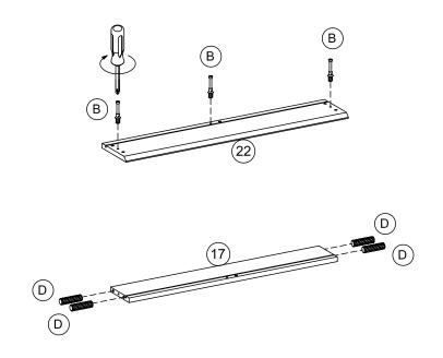
Attach cam-bolt (B) to front drawer (22) using screwdriver. Insert dowel (D) into rear drawer (17) as shown.
