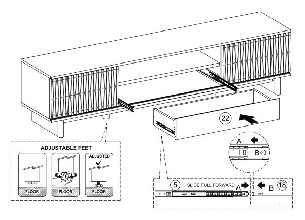
Insert the drawer into case assembly as shown. Adjust the leg until flat with floor.
