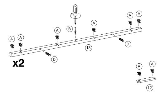
Attach cam-bolt (B) to bottom large support (13) using screwdriver. Insert cam-lock (A) and dowel (D) into bottom large support (13). Insert cam-lock (A) into bottom small support (12).
