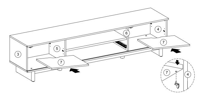
Insert adjustable shelf (7) into case assembly as shown.
