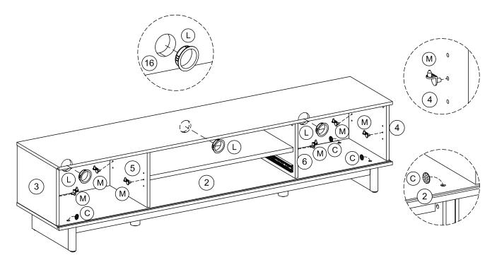
Insert cable holder (L) and shelf support (M) into case assembly as shown. Paste cam-sticker (C) to base panel hole as shown.
