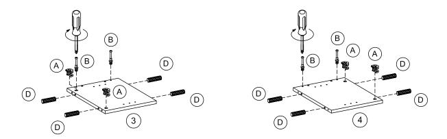
Attach cam-bolt (B) to left panel (3) and right panel (4) using screwdriver. Insert cam-lock (A) and dowel (D) into left panel (3) and right panel (4).
