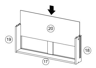
Insert Bottom drawer (20) to the drawer assembly as shown.
