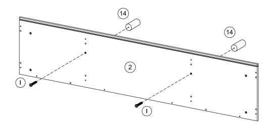
Attach leg (14) to base panel (2) using screws (I).
