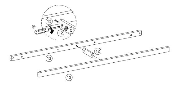
Attach bottom large support (13) to bottom small support (12) as shown. Turn the cam-lock (A) clockwise to lock using screwdriver, then paste cam-sticker (C).
