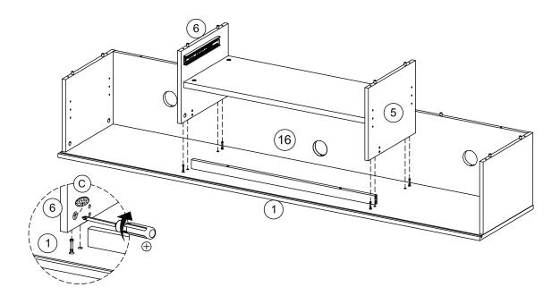
Attach assembly divider panel to the case assembly as shown. Turn the cam-lock (A) clockwise to lock using screwdriver, then paste cam-sticker (C).
