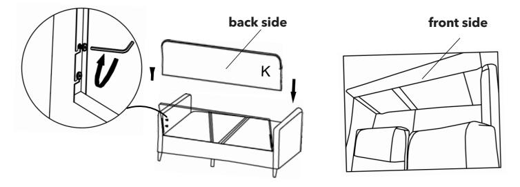
Make sure the back cover is put on the correct side
