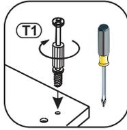
Tighten until shoulder is flush with panel. Do not overtighten or undertighten (see example below)
