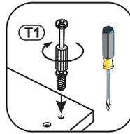
Tighten until shoulder is flush with panel. Do not overtighten or undertighten (see example below)
