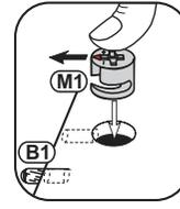
Tighten until shoulder is flush with panel. Do not overtighten or undertighten (see example below)
