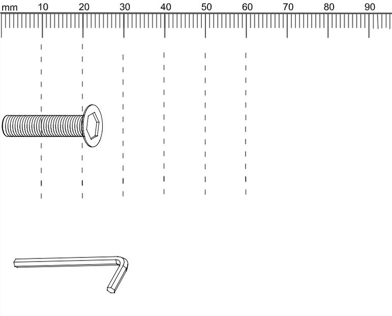
The image shows a technical drawing of two parts, A and B, with a ruler for scale. Part A is an M8\*25 screw, and Part B is a 5mm Allen key. The ruler is marked in millimeters from 0 to 90. Vertical dashed lines are drawn at 10mm intervals from 10mm to 60mm. Part A is positioned between the 10mm and 20mm marks, and Part B is positioned between the 10mm and 20mm marks.
