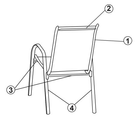
Do not tighten bolts until fully assembled.
