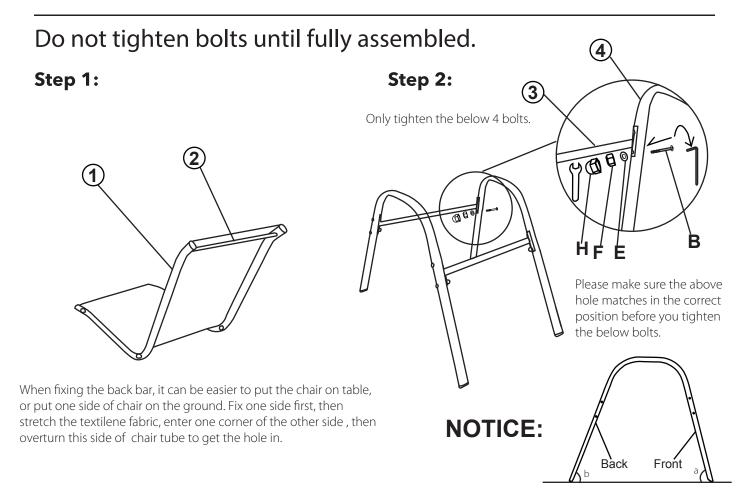
Put the 2 legs flat on the ground, you will see that the angle of 'A' is larger than the angle of 'B'. The back leg is more sloped that than the front leg.
