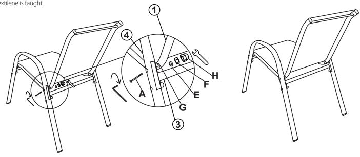
When fixing the seat to the other side of the legs, it can be easier to put the chair in a higher place, or lay the chair on the ground so you can see the fixings and stretch the textilene more easily.
