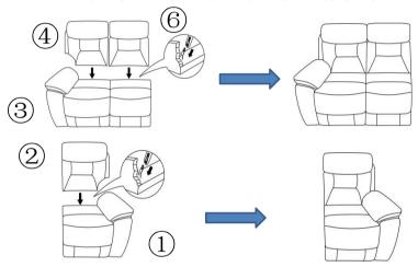
STEP2: ASSEMBLE UNITS FROM LEFT TO RIGHT BY HOOKING THE CLIP IN THE RIGHT SEAT BASE INTO THE LEFT SEAT BASE.
