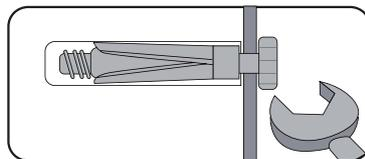
For use with heavier loads such as TV & Hi-fi Speakers and Satellite Dishes etc.
