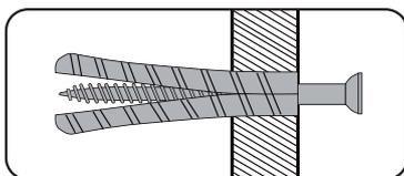
Generally aerated blocks should not be used to support heavy loads, use a specialist fitting in this case. For light loads, a General Purpose Plug can be used.
