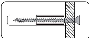
These come in various sizes and are made from plastic or sometimes wood fibre.
