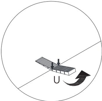
**The excess leveller can be broken off freely.**
