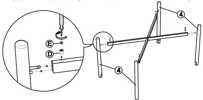
**IMPORTANT:** Hand tighten only to avoid damage to the legs.
