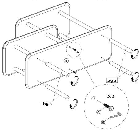
**IMPORTANT:** Hand tighten only to avoid damage to the legs \*DO NOT OVER-TIGHTEN.
