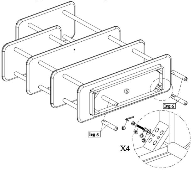
**IMPORTANT:** Hand tighten only to avoid damage to the legs \*DO NOT OVER-TIGHTEN.
