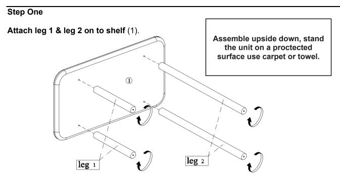
IMPORTANT: Hand tighten only to avoid damage to the legs \*DO NOT OVER-TIGHTEN.
