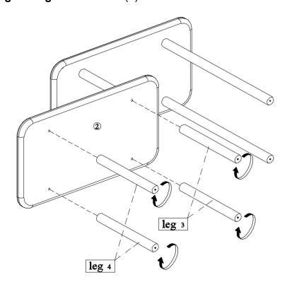
**IMPORTANT:** Hand tighten only to avoid damage to the legs \*DO NOT OVER-TIGHTEN. Page 5/14
