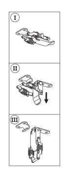
Release the two locks under the table top by pulling down the handle of the lock. Gently slide the top panels apart.
