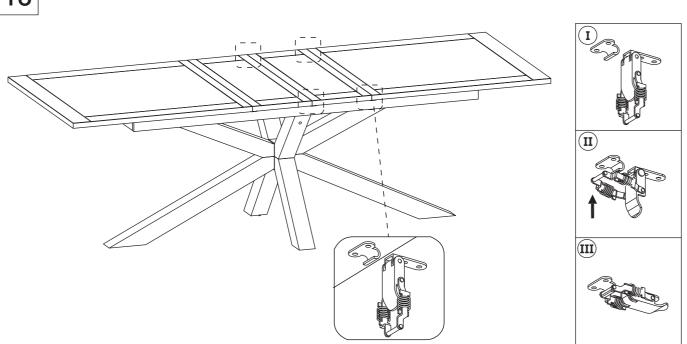
Fasten the four locks under the table top by placing the latch on each lock back to the hook, and closing the handle to lock.
