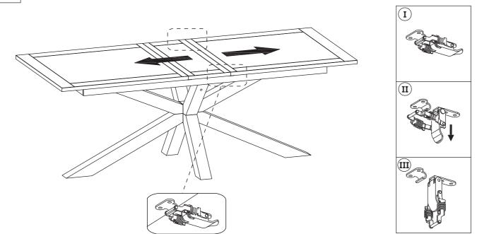
Release the two locks under the table top by pulling down the handle of the lock. Gently slide the top panels apart.
