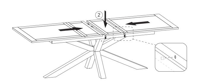
Place the remaining Add-On Panel (2) between the table top panel and the other Add-On Panel. Slide the panels back, making sure the pins are inserted into the guide holes of the panels.
