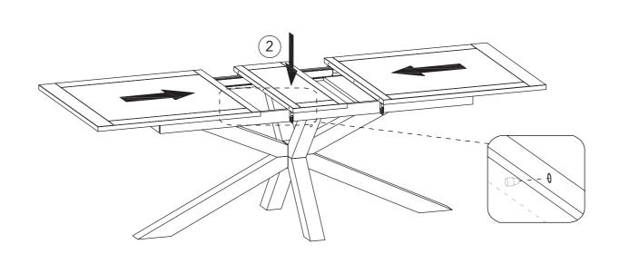
Place an Add-On Panel (2) between the two table top panels and slide the panels back, making sure the pins are inserted into the guide holes of the panels.
