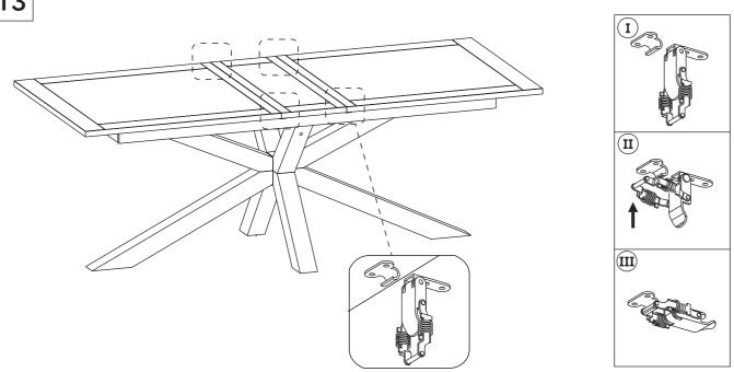
To lock the panels in position, place the latch on each lock back to the hook. Close the handle to lock.
