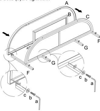
Install 2 x Centered Leg(G) using 8 x washers (c) and bolts (b) by allen key (a) as supplied.
