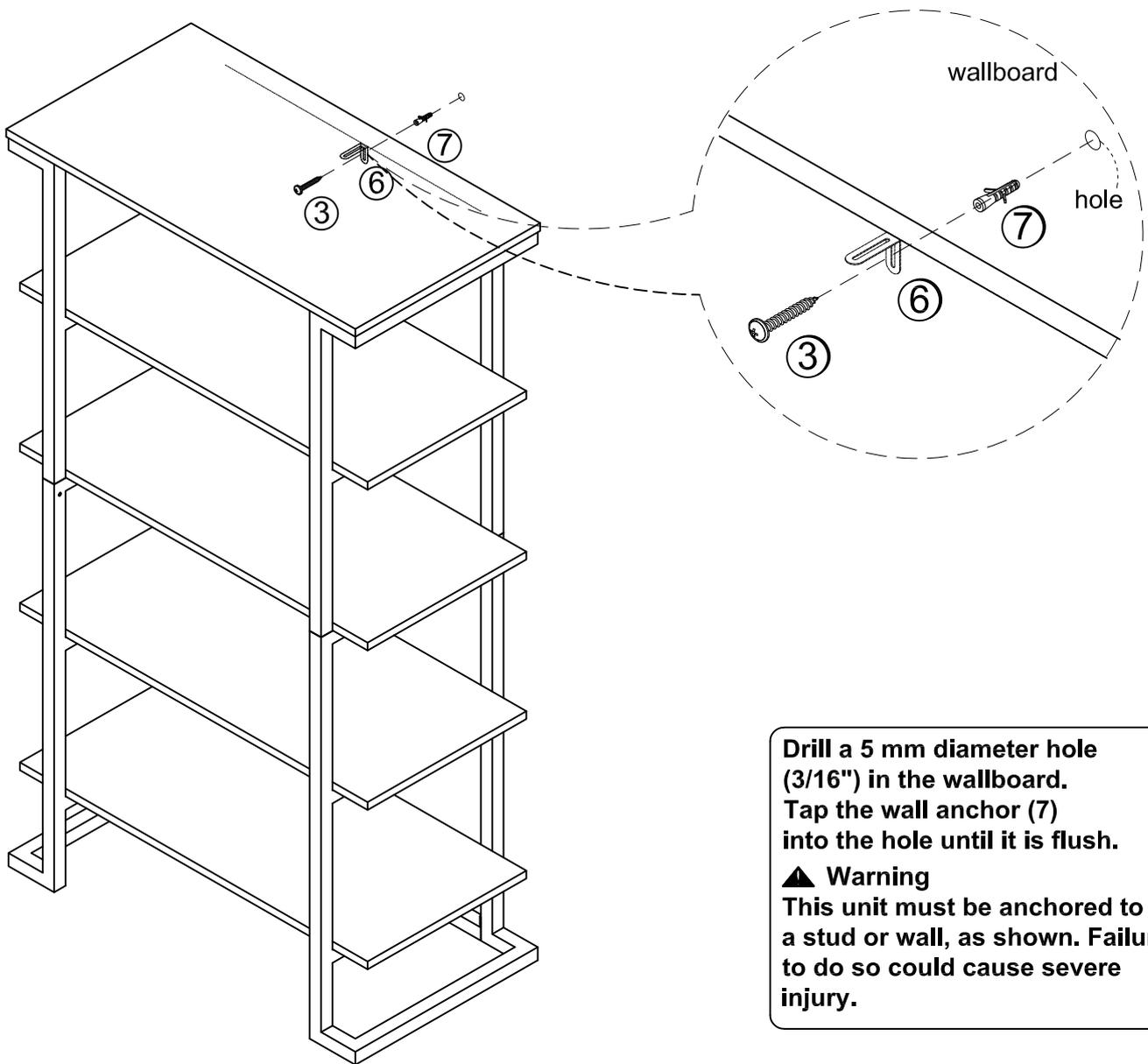
**Drill a 5 mm diameter hole (3/16") in the wallboard. Tap the wall anchor (7) into the hole until it is flush.**
