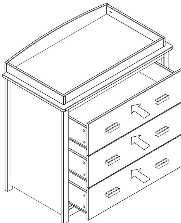
**WARNING! IN ORDER TO PREVENT OVERTURNING THIS PRODUCT MUST BE USED WITH THE WALL ATTACHMENT DEVICE PROVIDED.**
