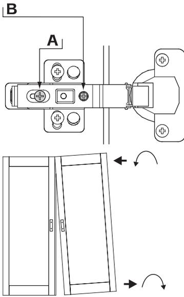
Adjusting the gap between the doors. Loosen screw 'A' slightly. Turn Screw 'B' clockwise to move the door away from the side, turn anti-clockwise to move the door towards the side. When gap is equal tighten screw 'A'.
