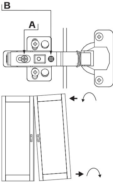
Adjusting the gap between the doors. Loosen screw 'A' slightly. Turn Screw 'B' clockwise to move the door away from the side, turn anti-clockwise to move the door towards the side. When gap is equal tighten screw 'A'.
