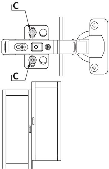
Adjusting the height of the doors. Loosen screws 'C' then slide the hingeplates up or down until the doors are even then tighten the screws.
