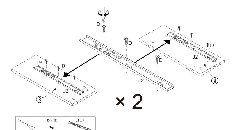
**Step 5:** Need to assemble drawer runner in the correct pilot hole as the diagram indicates.
