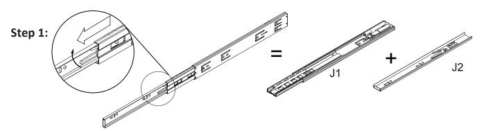
Need to assemble drawer runner in the correct pilot hole as the diagram indicates.
