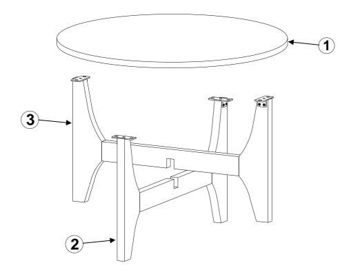
**Step 1:**Attach Leg frame (2) into Leg frame (3) by using Bolts (A) with Spring Washer (C) and Flat Washer (D) then fastening all Bolts securely using Allen Key (E).
