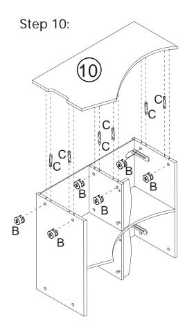
Put all the screws bolts/nuts, wood dowels and the back panel in acurrate position and keep all the screws bolts / wooden dowels align with holes of body when assembling. then pat the side panel slightly into the right postion, then lock the cam nuts.
