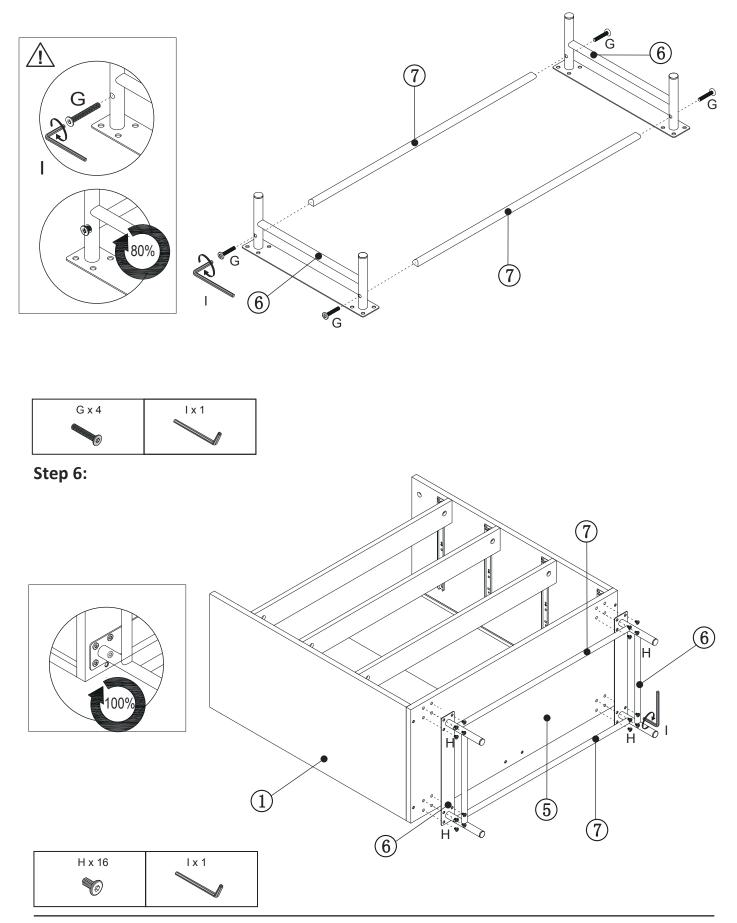
**Step 5:** Do not tighten the screw until you attach the metal frame onto the bottom panel.
