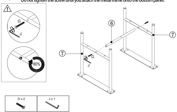
**Step 7:** Do not tighten the screw until you attach the metal frame onto the bottom panel.
