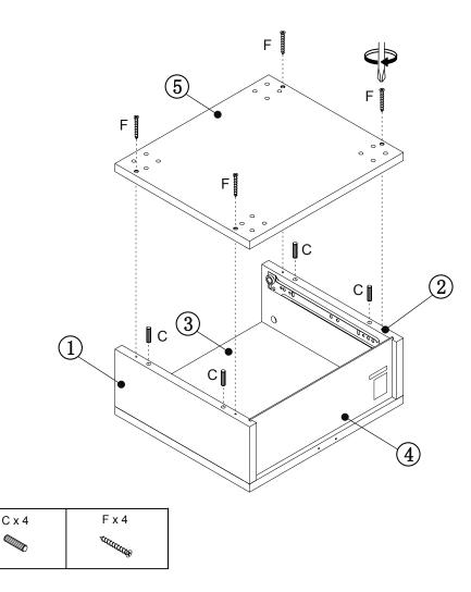
Step 6: Do not tighten the screw until you attach the metal frame onto the bottom panel.
