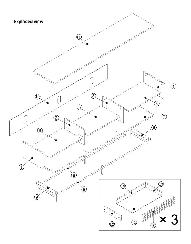
Need to assemble drawer runner in the correct pilot hole as the diagram indicates.
