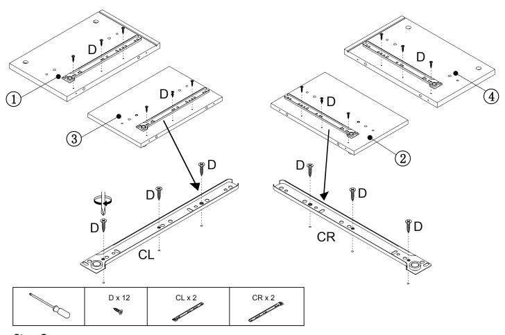
**Step 2:** Need to assemble drawer runner in the correct pilot hole as the diagram indicates.
