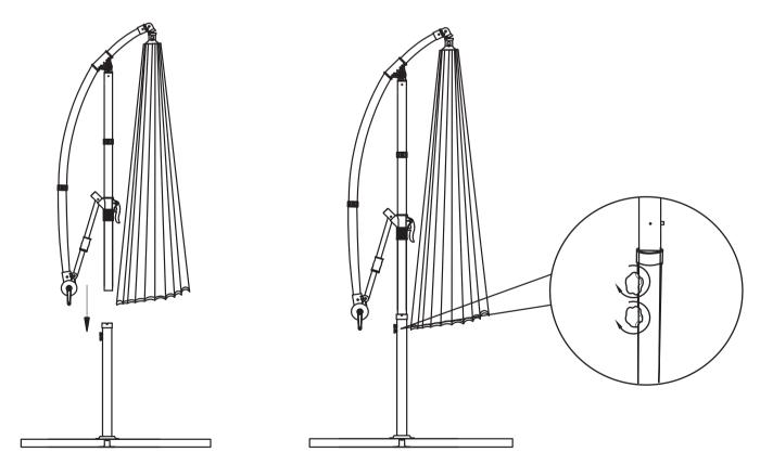
Make sure the two knobs are fully locked.
