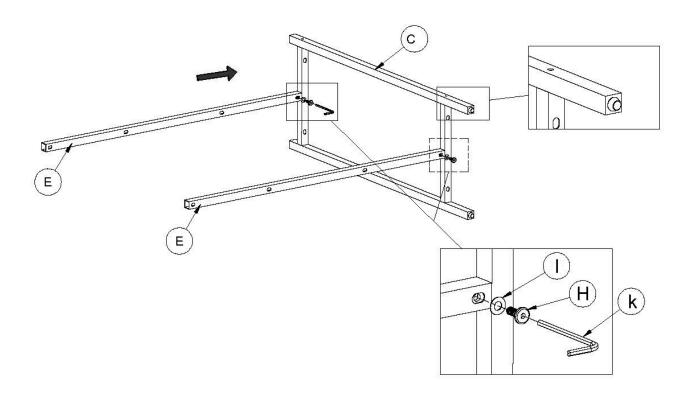
**IMPORTANT:** To avoid damage to the parts, tighten fixings by hand only.
