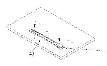
Need to assemble drawer runner in the correct pilot hole as the diagram indicates.
