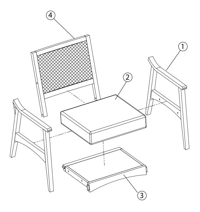
Please place a sheet or cloth on the floor to prevent damage to the unit when assembling and do not fully tighten the bolts before final assembly.
