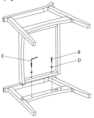
Step 4: Align the back panel (4) to the leg panel, secure using bolt (A) and washer (D) using allen key (E).
