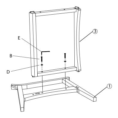
Step 3: Align the 2nd leg panel by fitting the blocks on seat panel (3) into the slotted holes, secure using Bolts (B) and washer (D) - tighten with Allen key (E). and do not fully tighten.
