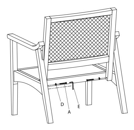
Step 5 : Align the top holes in the back panel (4) with the holes at the back of the arms (1) and secure with bolt (C) and washer (D) fully tighten all bolts using allen key (E).
