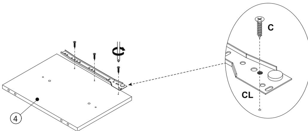
Need to assemble drawer runner in the correct pilot hole as the diagram indicates.
