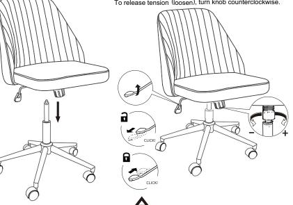
Press the lever up to adjust seat height Pull out the lever to unlock rocking mechanism
